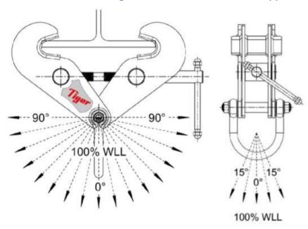
No deration up to 90° has been established for BCF model clamps and applies only for overhead beam attachments. It does not apply when used for lifting beams. Our BCF clamp has been specifically designed for this purpose.
